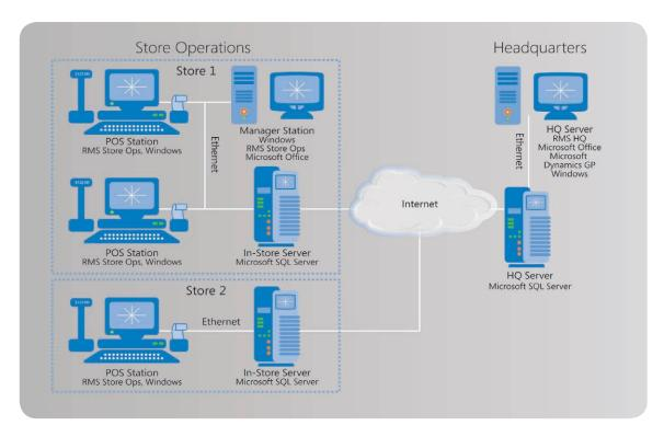
A typical deployment of Microsoft Dynamics Retail Management System in a two-store scenario—one store with multiple lanes. A local area network (LAN) connects Microsoft Dynamics Retail Management System Store Operations installations across checkout lanes or POS stations within the store, and an Internet connection connects the stores to a head office running Microsoft Dynamics RMS Headquarters For details on additional store-level configurations, contact your Microsoft Certified Partner...
